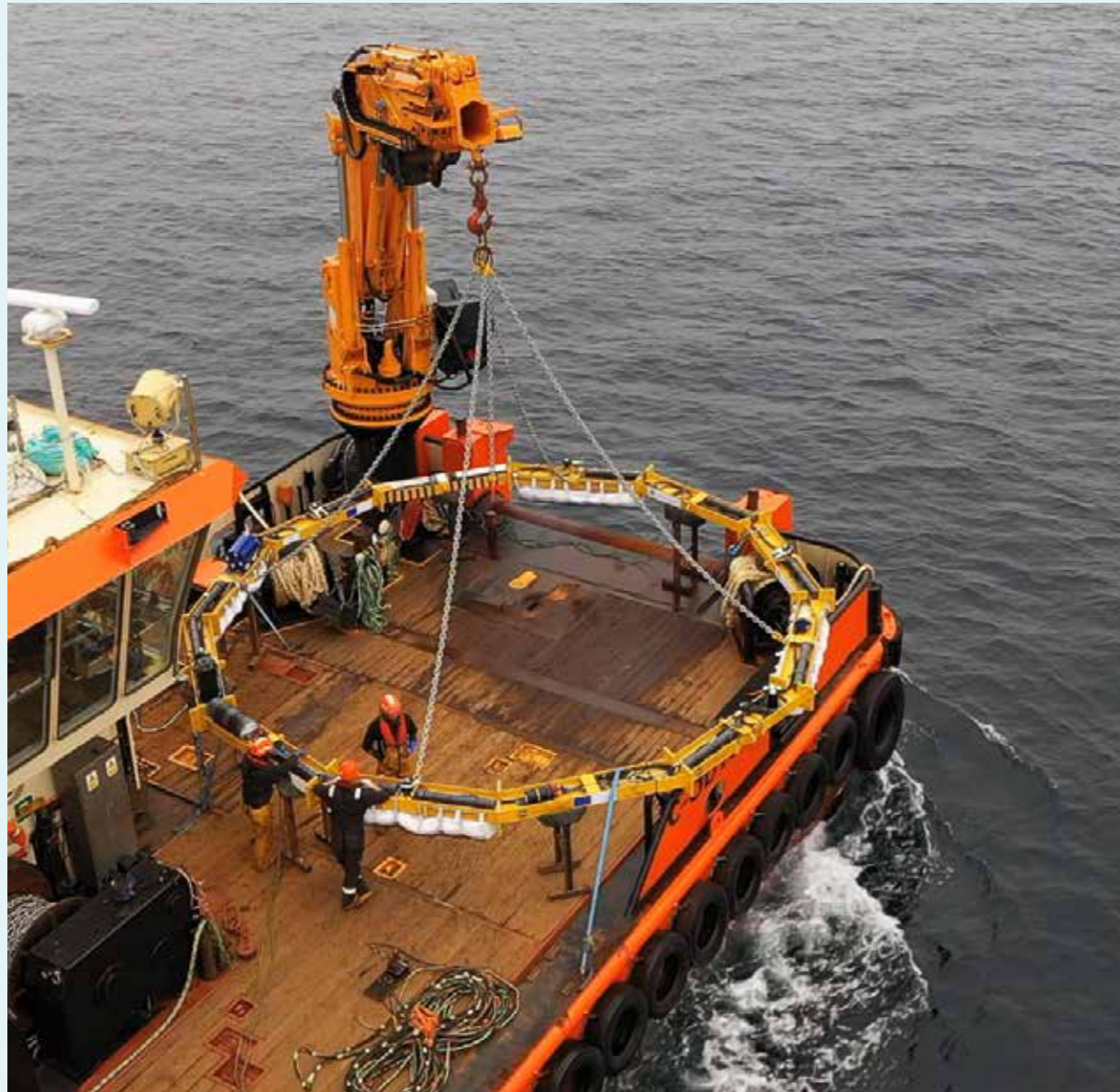
RealTide Advanced Turbulence Sensor (Source: University of Edinburgh & EMEC)
